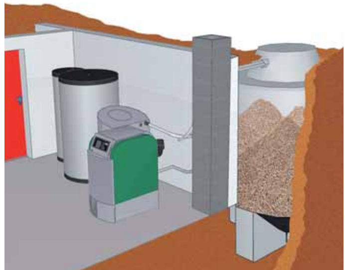
Fuel transport with suction system out of an underground bunker.
