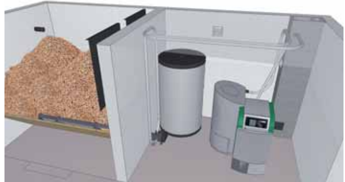
Fuel transport with a screw in the storage room and suction system to the boiler.
