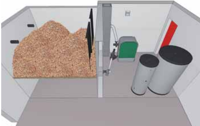
Fuel transport with flexible auger system and transfer hopper.
