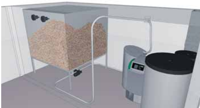
Fuel transport with suction system out of a bag silo.
