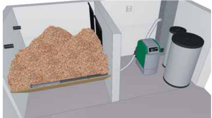
Fuel transport with flexible auger system.
